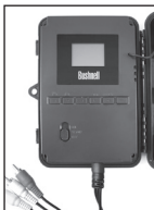
Cable from "A/V Out"
